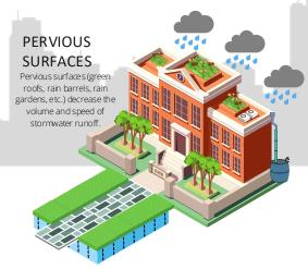
Trees, gardens, and other technologies are designed to help reduce stormwater runoff by absorbing or storing it for slow release. The vegetation and soil also act like a filter, trapping oils, heavy metals, dirt/road grime, and trash - preventing it from entering our waterways.
