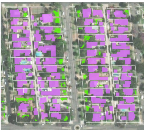
Parcel analysis scaled up across neighborhoods. Green areas show opportunities for bioretention.
